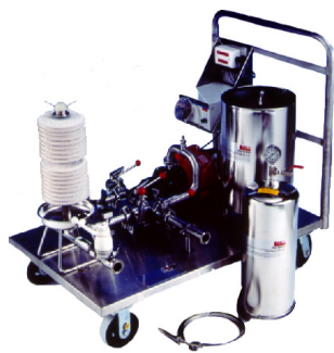
Figure 46 - Zeta Plus™ filter housings can be skid mounted for even more flexibility.
