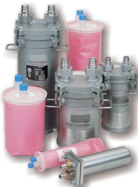
Figure 26 - CUNO™ CTG-Klean System: The filter pack provides the barrier between the ink and the housing, reducing change-out times and operator exposure.
