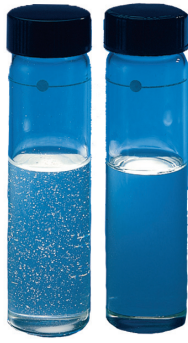
Figure 9 - Resin clarity specifications are often based on visual, Gardner, or APHA techniques. Regardless of the inspection method, 3M Purification has the solution. Shown above is single pass resin haze removal by Zeta Plus™ filters (before left, after right).
